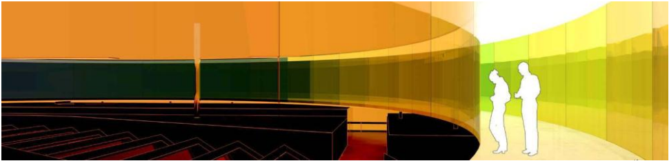
Figure 2: View of the inner appearance of the glass walls, no structural elements are in the inner and outer walls except the curved glass panes
